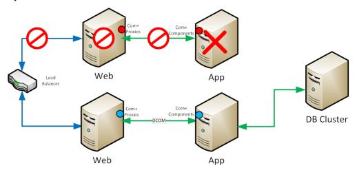
This requires that the load balancer/failover router be capable of monitoring the health of each channel as a whole and not just the web server that sits at the front of it.
