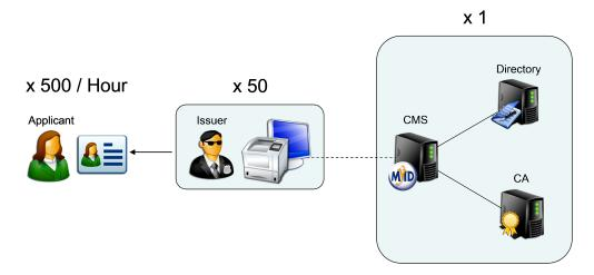
In the example above a simple single server MyID architecture (web server, application server and database all installed on the same machine) was used. MyID was connected to an Active Directory and a CA.
