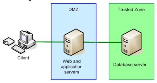
For high security environments, a three-machine architecture may be used:
