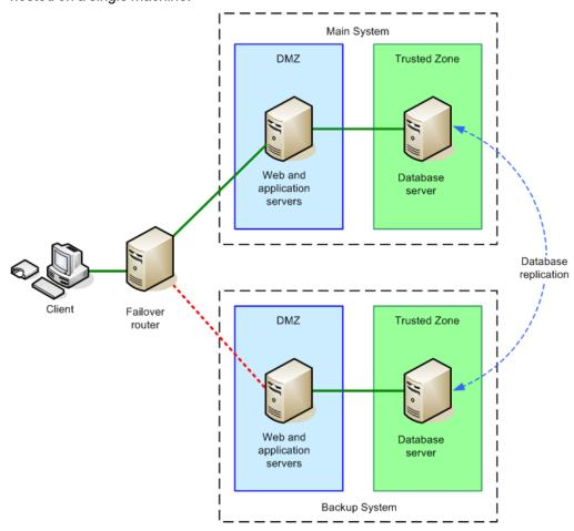
This solution provides resilience against both component and network failure. It is common to locate the main system and backup system on different networks, hosted on different sites, to protect against total infrastructure failure at on site, such as a major power failure.
