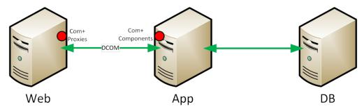
The proxies that run on the web server must be derived from the instance of the components on the individual application server that they are paired with.
