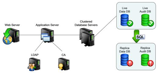
In the example above Microsoft SQL Server Clustering was used to provide failover only, no load balancing was used. In addition the audit database was split out from the main operational database.
