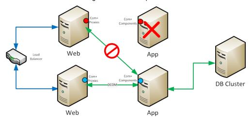
This is because the proxies on the web server in the top channel are not paired with the application server on the second channel. That is, the communications from top channel web server to the second channel application server will not work.
